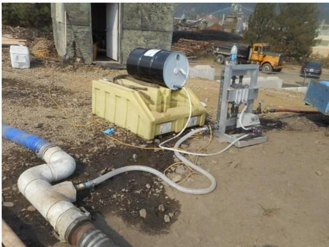
WaterSolve provided the polymer make-down system and the Solve 151 flocculent which was injected into the 6" piping system going to the Geotube® containers.
