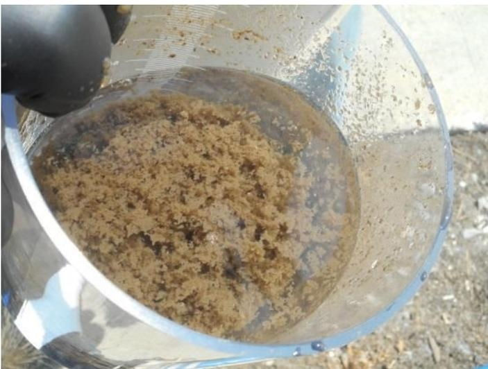
The WaterSolve technician trained the operators to attain a floc that looked like this when adjusting the dose of polymer.
